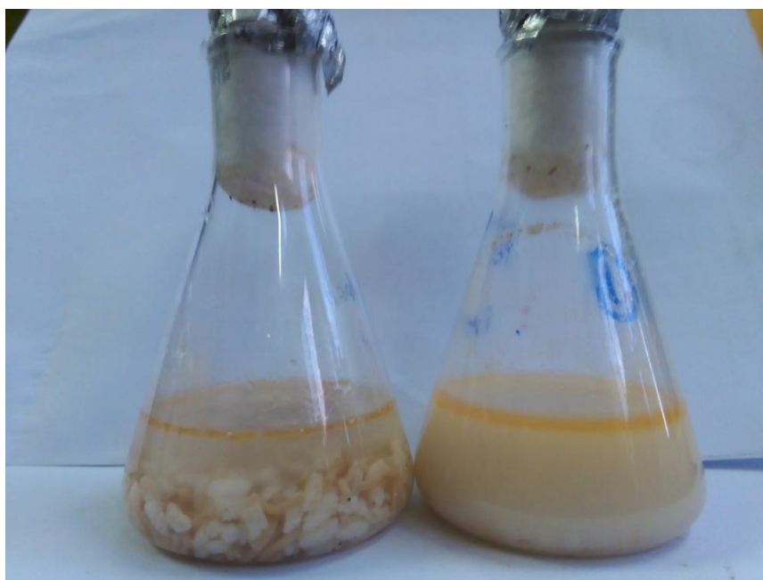
Figure 2: Biodegradation of cooked rice grains by \alpha -amylase enzyme. The left flask is untreated rice grains and the right flask is the treated rice grains.
